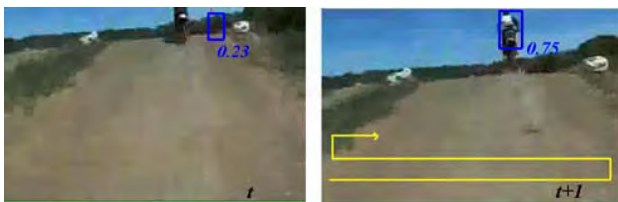
Fig.7. If previous frame's trajectory is not good (left image with the confidence 0.23), the detector performs global search by sliding window to find best object location (blue bounding box with the confidence 0.75).
